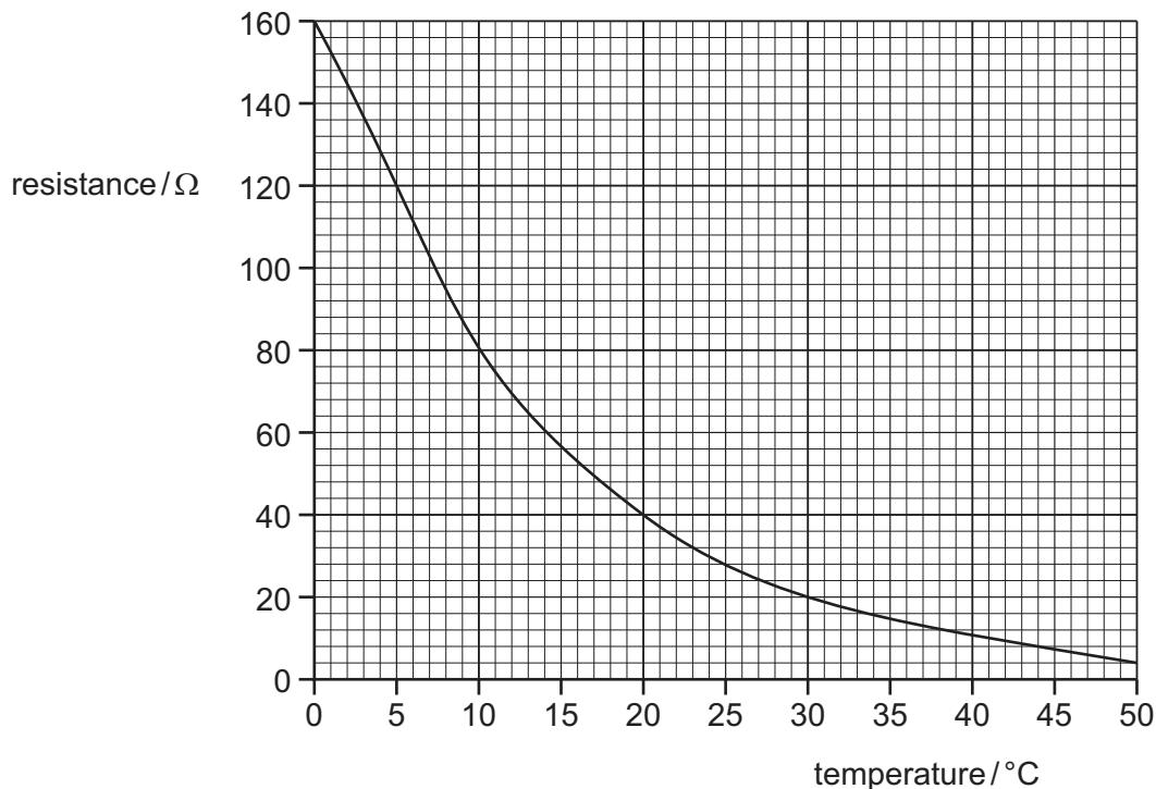
The thermistor is at a temperature of  $10\text{ }^{\circ}\text{C}$  and is connected in series with a fixed resistor of resistance  $20\text{ }\Omega$ .
