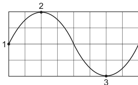
What are possible angles between the plane of the coil and the magnetic field direction at the times represented by points 1, 2 and 3?
