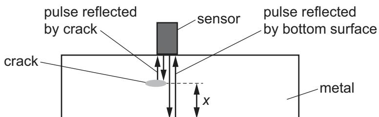
The reflection from the crack is received back at the sensor  $1.0 \times 10^{-5}$  s after the pulse is sent out.
